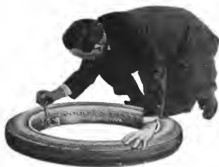
Fig. 6—Locking (or unlocking) the rim
